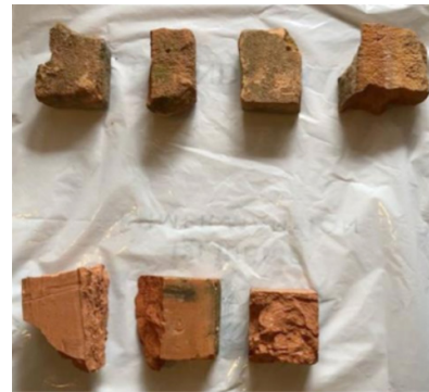
Picture 1. Collected Brick Samples (up-bricks from 10thCentury/ down-currentlyusedbricks)
